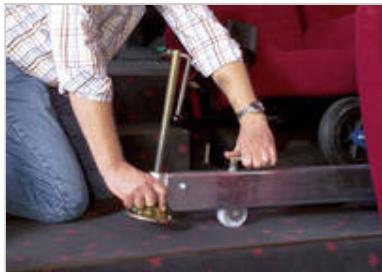
**5. After the desired position has been reached, the rollers are released and the Movielift is secured with the aid of its support feet.**
