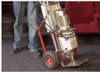
**7. The 230V drive of the Movielift is mounted on a separate elevating truck and can be placed at a distance of maximum 10 m next to, in front of or behind the Movielift.**
